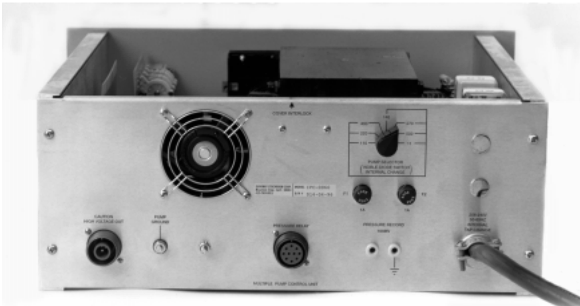
Figure 5: Rear Control Panel
